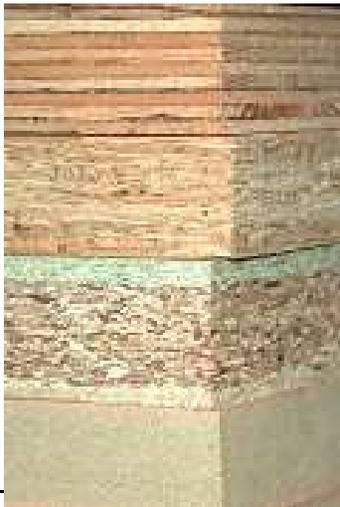
**Products:** Wood-based panels in the form of solid wood panels, LVL, plywood, OSB, particleboards (chipboards) either resin- or cement-bonded, wet process fibreboards (hardboards, medium boards, softboards) and dry process fibreboards (MDF) for use in construction. They may contain chemical agents to improved their reaction to fire and their resistance to biological attack, e.g. by fungi and insects.
